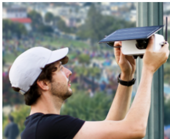
Figure 6 - Clarity continuous monitoring unit mounted to a pole
