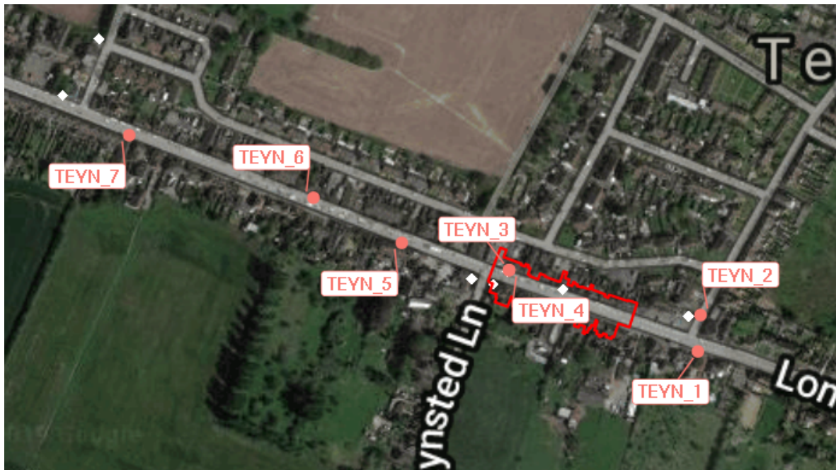
Figure 4 - Proposed locations (approximate) for NO 2 diffusion tube monitoring in Teynham/Lynsted. White diamonds show the existing local authority monitoring locations.
